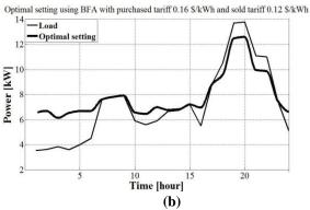
Figure 5 Effect of sold price on microgrid optimal operation
